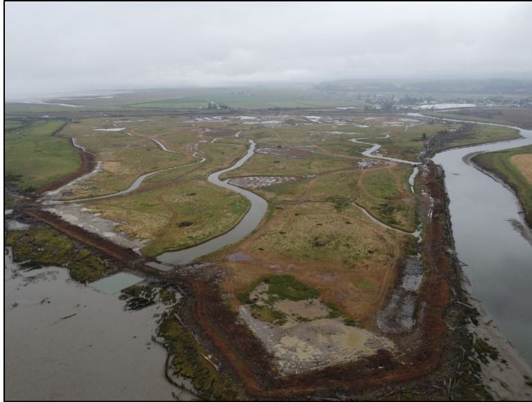
The WDFW drone captured some good photos of the Leque site, including this one looking North over the restoration area. After the dikes are removed in October, the channels will be connected to the surrounding river and marsh.
