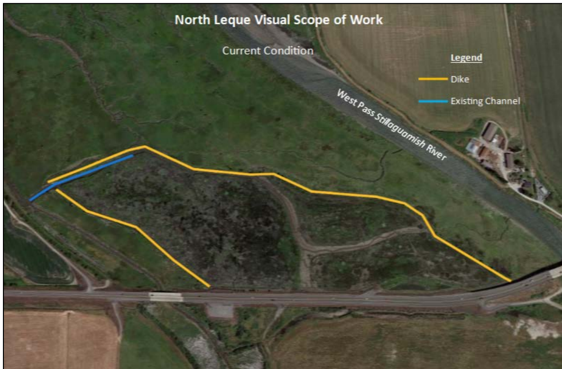
There is currently a single opening in the dike at North Leque Island where a tide gate failed over 10 years ago
