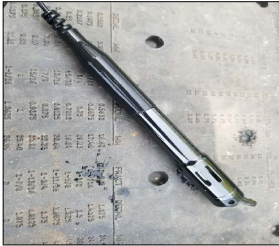
This is a level logger device. Several of these are deployed in and around Skagit Bay to help us understand how water levels and salinity change throughout the year under different river level and tidal conditions.
