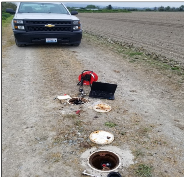
Downloading level logger data in a pair of wells adjacent to the Headquarters Unit
