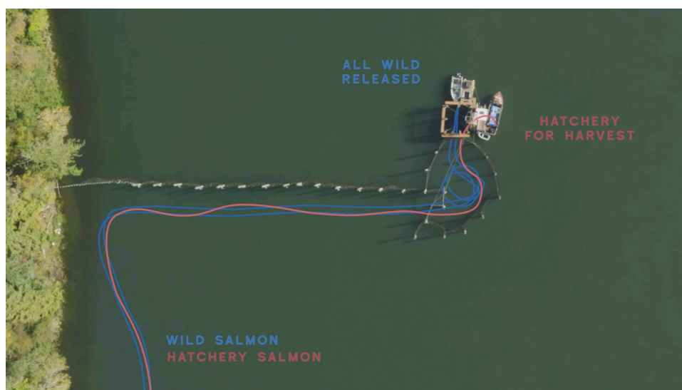
Video 1. Vid. 1. An experimental fish trap in Cathlamet Channel, WA funnels returning adult salmonids from the lead wall to a sorting compartment in 2019. In the final moment of capture, the catch can be brailed or funneled passively to the sorting compartment for data collection and release, or selective harvest. A video clip is available online. Supplementary material related to this article can be found online at doi:10.1016/j.fishres.2022.106495 .
