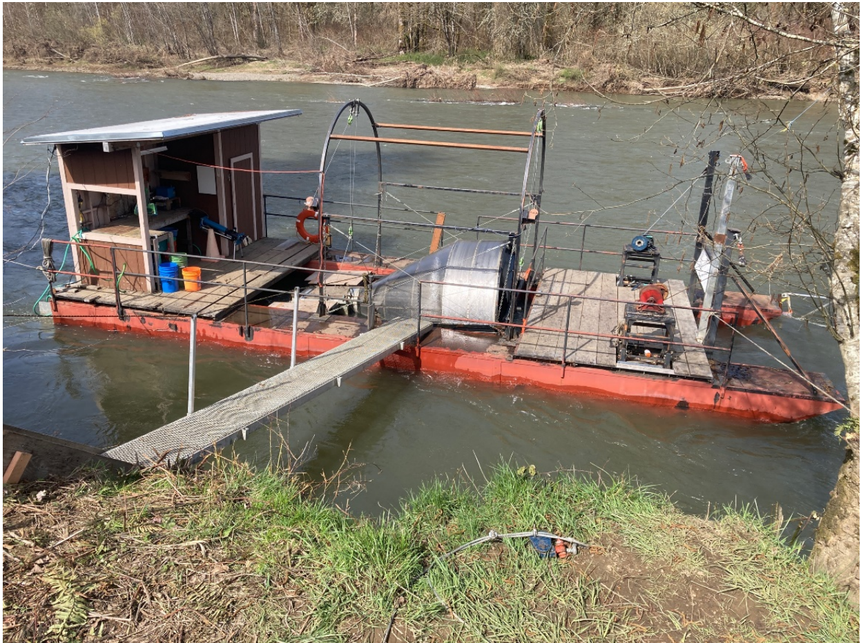
Figure 5: Rotary screw trap used to estimate juvenile steelhead abundance originating upstream of river mile 52 on the Chehalis River showing cone, livebox (covered), and floating pontoons. (Photo: D. Olson)
