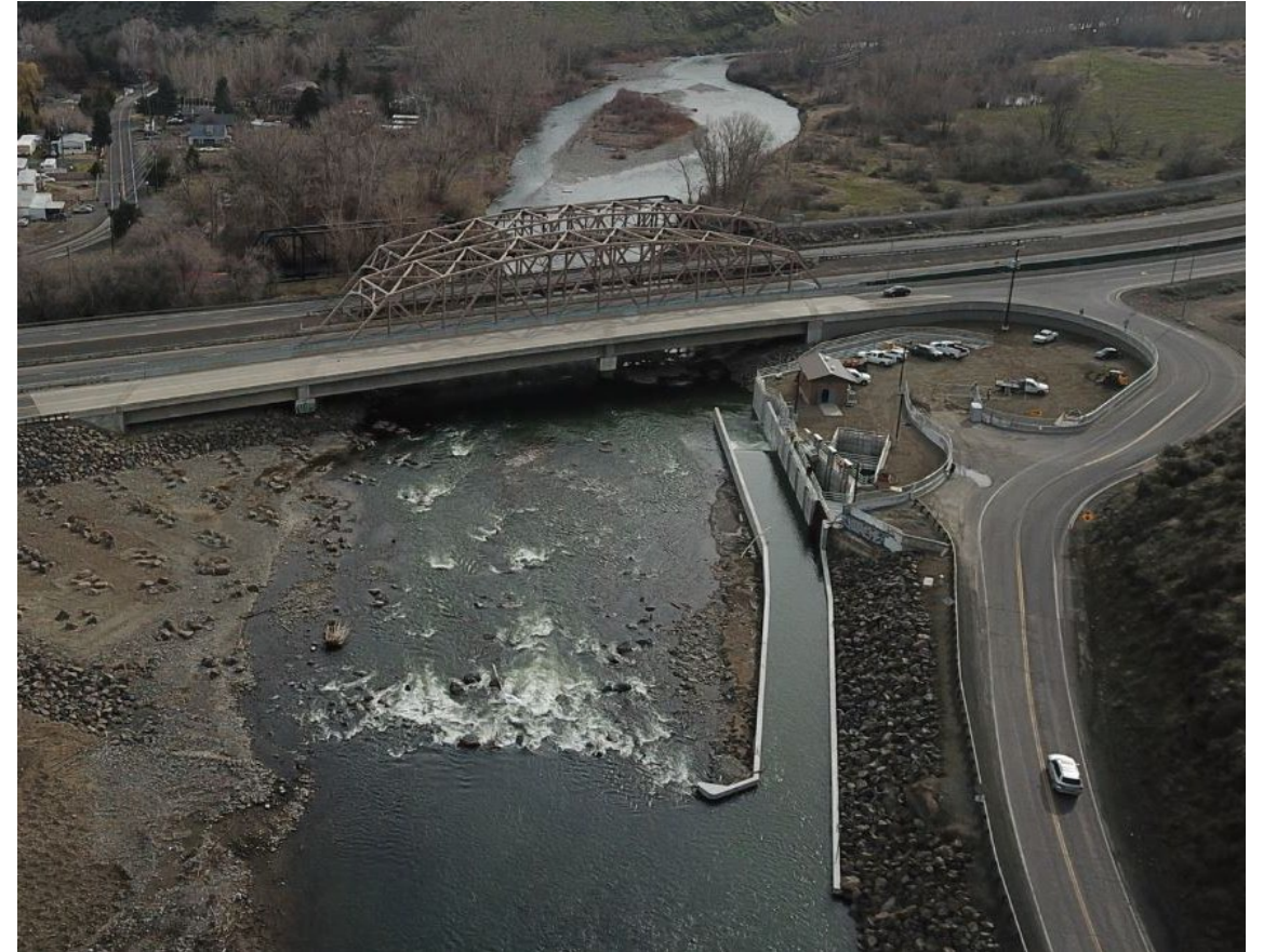
After: Fully passable crest based roughened channel. Photo Courtesy of Mike Shane, City of Yakima
