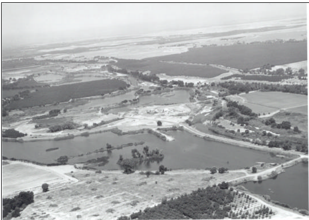
Figure 31. Oblique aerial view of the Ruddy reach of the Tuolumne River showing multiple floodplain gravel pits and the river channel, which itself flows through former in-channel pits (Photo by Kondolf 2000).
