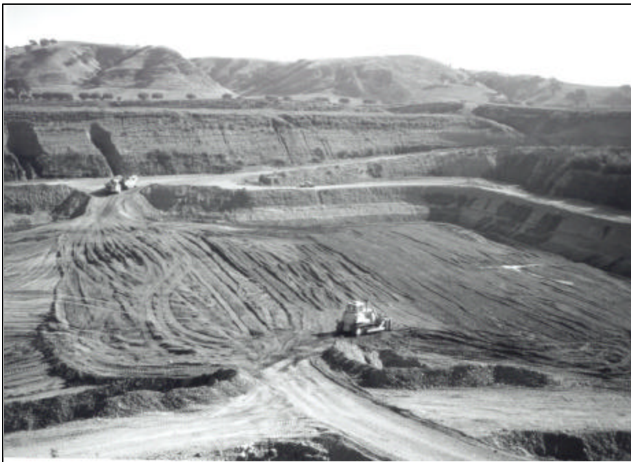
Figure 19. Gravel pit dewatered by pumping, Alameda Creek at Sunol, California (Photo by Kondolf 1990).
