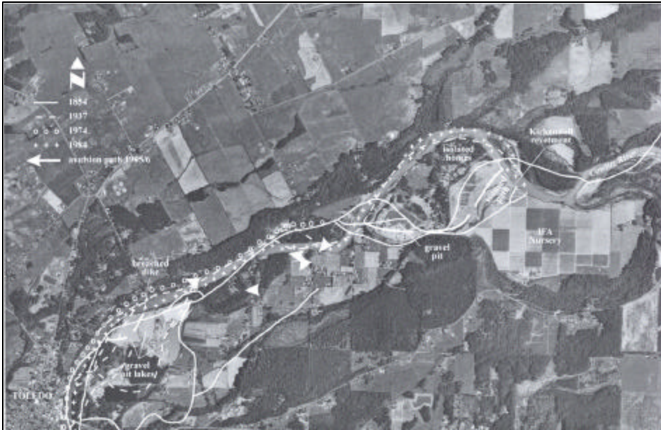
Figure 34. Vertical aerial photograph (July 1996) of the Cowlitz River from Toledo, Washington, upstream, annotated to show flow paths of the 1995 and 1996 floods (Reproduced from Norman et al. 1998, used by permission).
