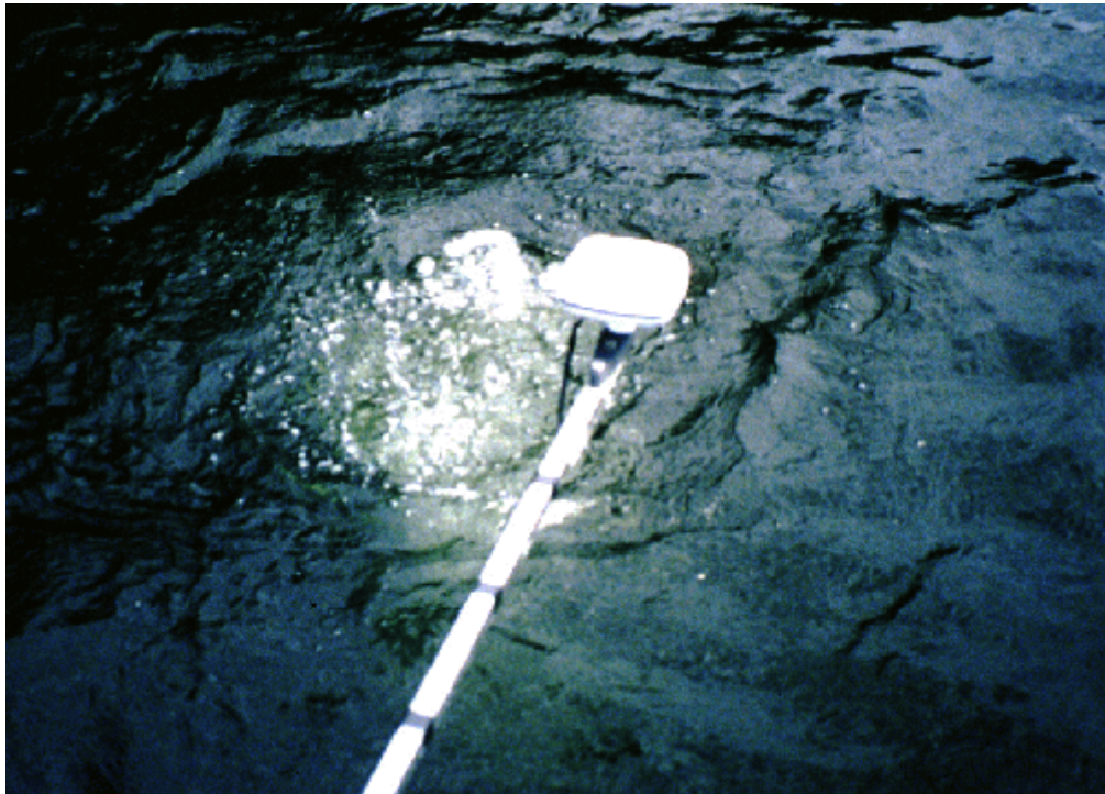
Figure 9. The start and end points of each transect, and all observation points in between, were located by positioning a GPS antenna over the exhaust bubbles of WDFW divers stationary on the bottom (photo by Karl W. Mueller).
