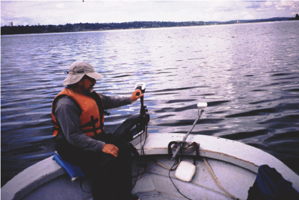
Figure 11. WDFW surface tender positioning support vessel and GPS antenna over divers' exhaust bubbles during the deep transect off Seward Park (Bailey Peninsula), Lake Washington (photo by Karl W. Mueller).
