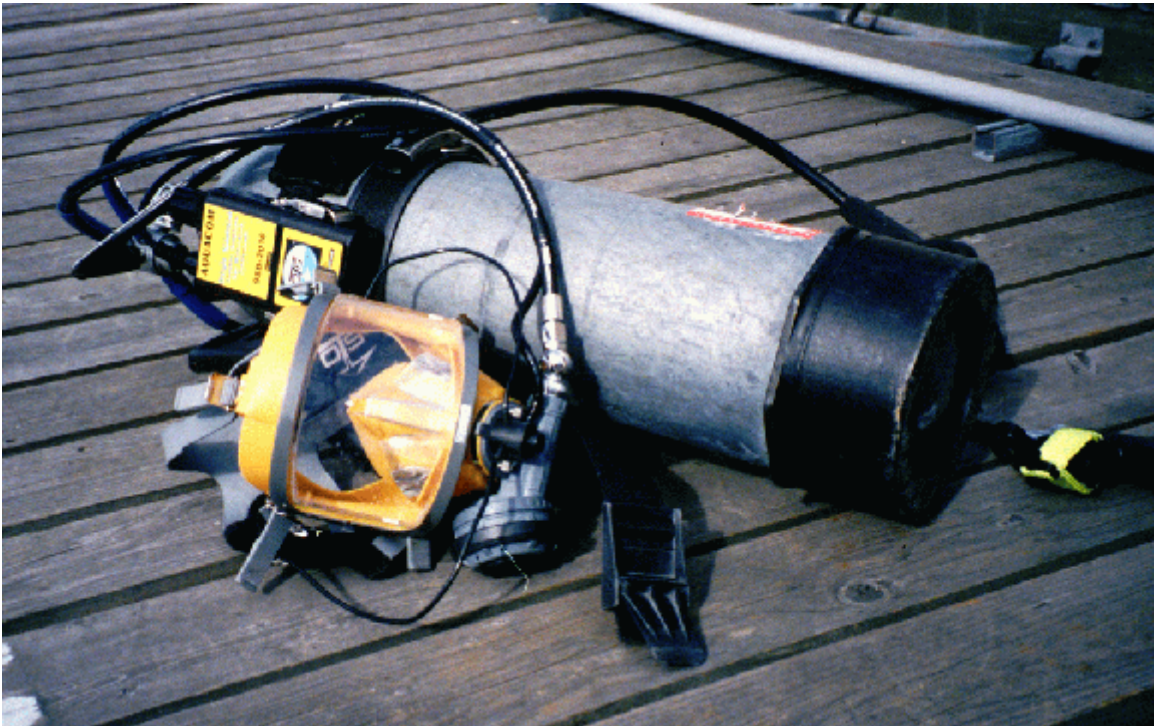
Figure 12. Full face mask underwater communication system used in dive operations at Lake Washington and Lake Union during spring and summer 2000 and 2001 (photo by Karl W. Mueller).
