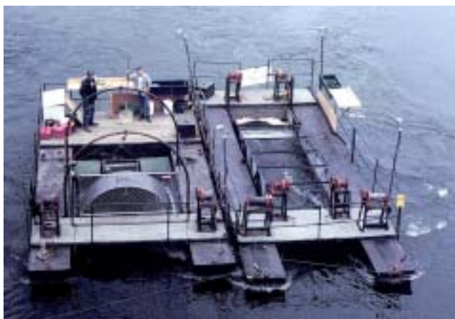
Smolt traps like these are a common sight on the Skagit River, where WDFW has used them to measure freshwater production of juvenile salmon since 1990.
