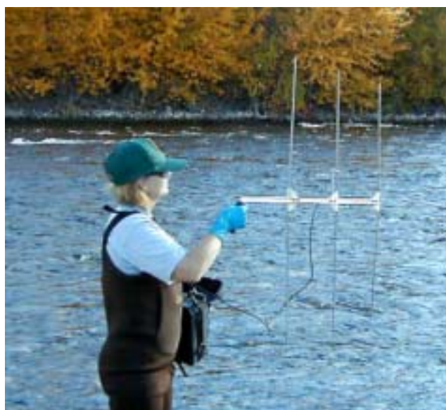
Using a radio telemetry device, a WDFW biologist monitors the migration of tagged adult salmon upstream.
