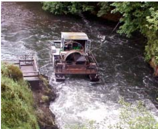
A screw trap measures downstream migration of chinook and coho salmon on the Deschutes River.
