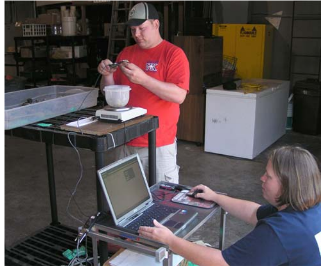
Figure 1-3. WDFW resource technicians use a laptop computer to automate the entering of clam measurement data from a digital caliper and scale. (Dale Gombert)
