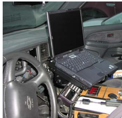
Figure 3-9. Mobile computer mounted in vehicle of WDFW Enforcement officer.
