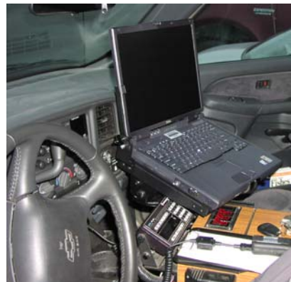
Figure 3-8. Mobile computer mounted in vehicle of WDFW Enforcement officer.
