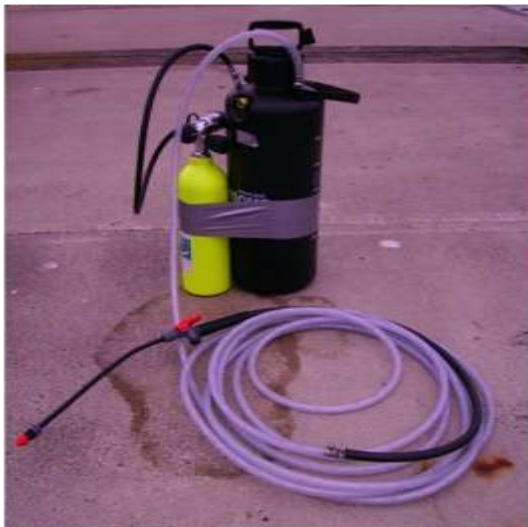
Figure 7. Hose end sprayer pressurized with SCUBA cylinder used for in situ application of 30% acetic acid.
