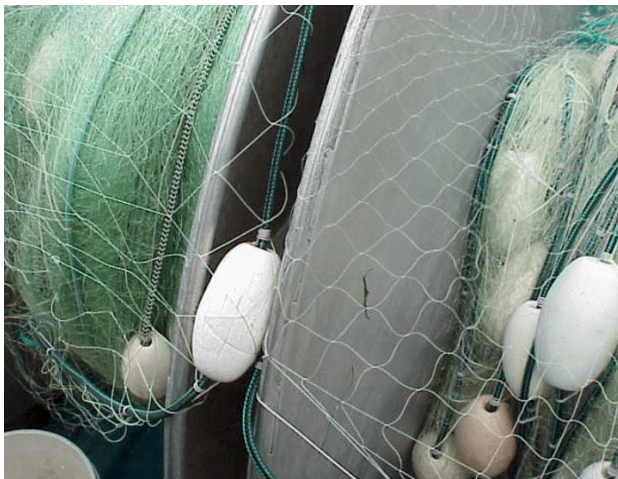
Figure 1: Comparison between the conventional monofilament gill net (left) and the multi-strand tangle net (right). The mesh size of a conventional net is chosen to fit the target species so that the target fish is caught around the gills and body. Fish caught in this way are often injured or killed in the net because they are unable to continue to respire. In contrast, the mesh size of the tangle net is designed to capture the fish around the face to prevent injury and to allow continued respiration. Fish caught live can be either kept for harvest, or released.
