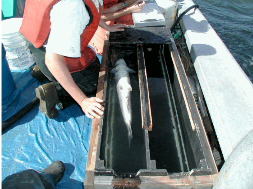
Figure 3: Recovery box used to revive fish stressed by capture. The box is designed so that a continual flow of fresh water is directed at the fish's face. Fish may need more than an hour in the box before they are fully recovered, and will begin to swim. This box had a ruler built in so that the fish did not need to be removed from the water for measuring. When the fish was ready to be released, it was gently lifted out of the box and placed overboard.
