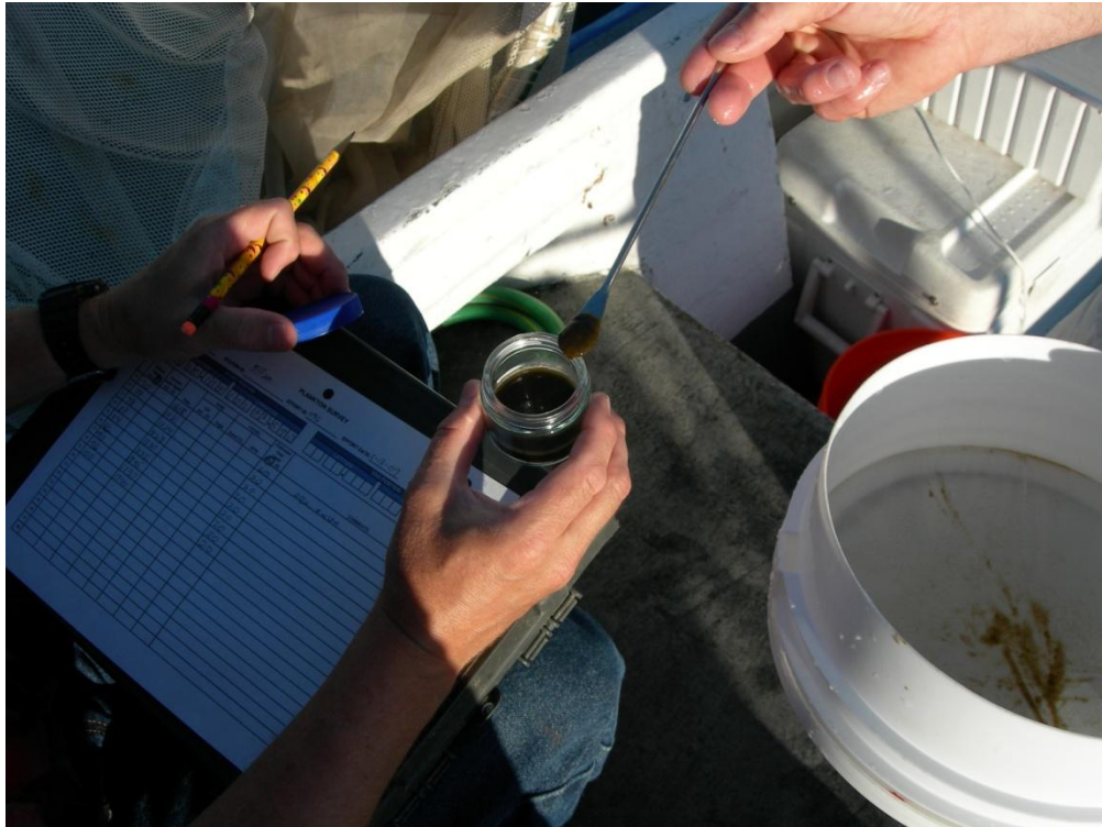
Figure 5. Collection of particulate organic matter (POM) paste concentrated on a 20- \mu m sieve.
