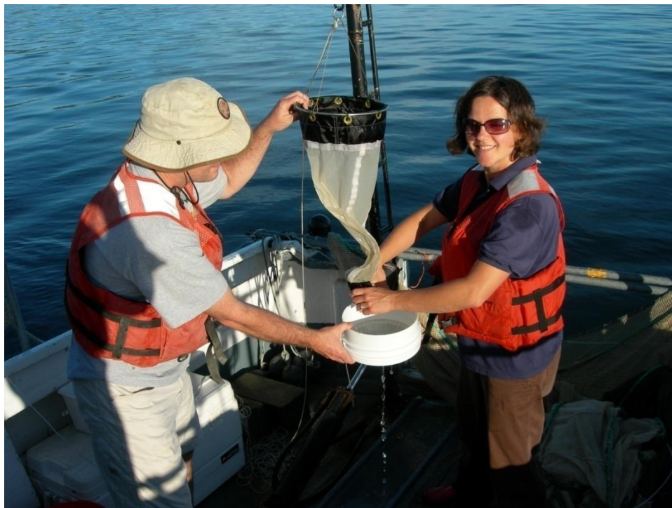
Figure 4. Conical plankton sampling net (20 \mu m mesh pore size) used to sample particulate organic matter.
