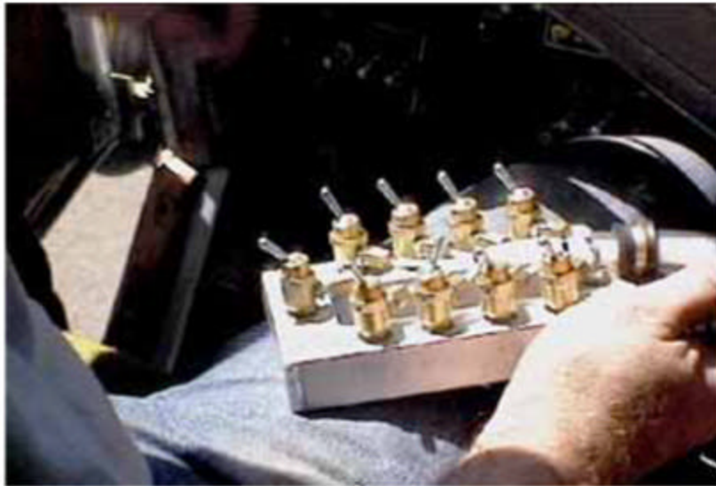
Plate 52. Release of tanks 1 through 8 places fry and water in the 9th tank, which is controlled by the far left toggle switch. The 9th, or posterior "ready" tank is dumped when in position over the target lake. Photo by Soloy Corporation.
