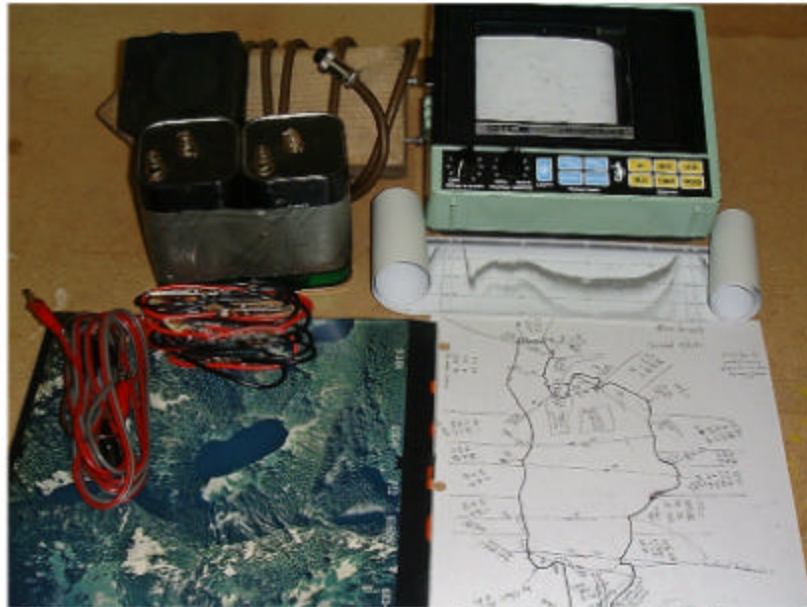
Plate 10. Essential components for bathymetric mapping using a chart recorder include a transducer that can be towed behind the raft, a pair of 6-volt batteries that can be wired in series to produce 12 volts, a high quality aerial photo of the area, and the base map outline to establish transect end points. Snoqualmie Lake in the Middle Fork Snoqualmie River drainage is shown on the base map.
