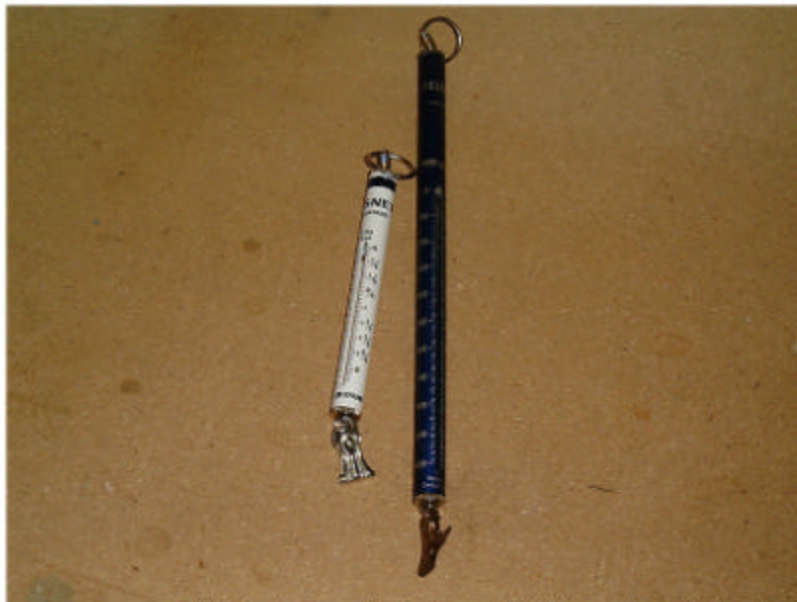
Plate 27. Precise measurements of fish weight can be obtained with light, easily packed spring scales. The blue scale, about 9 inches long, can be read to one gram.
