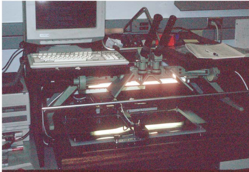
Plate 8. A stereo analytical plotter utilizes two adjacent aerial photos that have been corrected for parallax, and which are controlled, or linked to known GPS coordinates. The system has a high degree of precision; a white dot viewed through the optics corresponds to about 30 feet on the ground. Digitized lake polygons, or attributes such as islands, are logged in files created on the linked computer to enable calculation of metrics such as lake surface area, shoreline length, etc.
