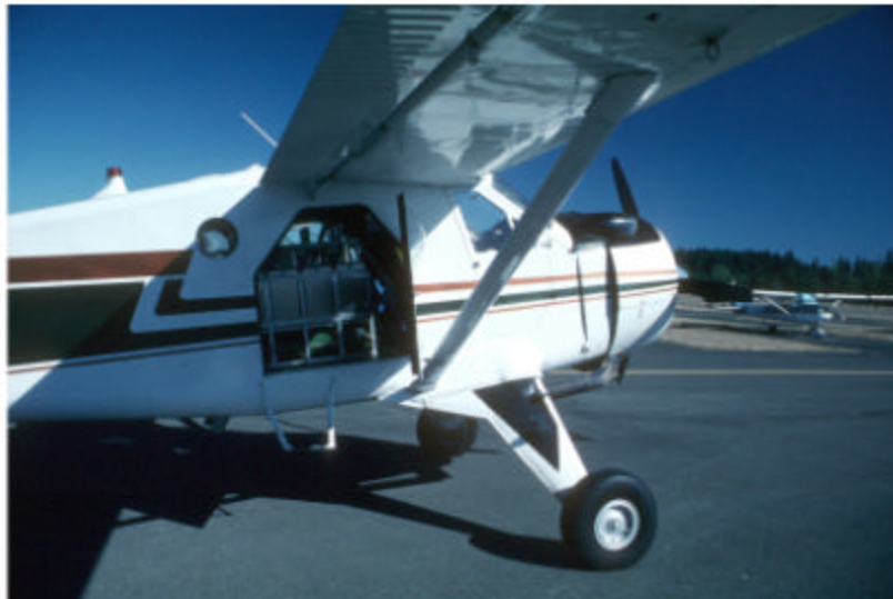
Plate 51. The drop tank was designed for the deHavilland Beaver. The drop tube is seen exiting the camera port to the left of the step, and below the fuselage port-hole. The individual tanks are loaded from both sides of the plane. Darrington airfield, (30 September 1998)
