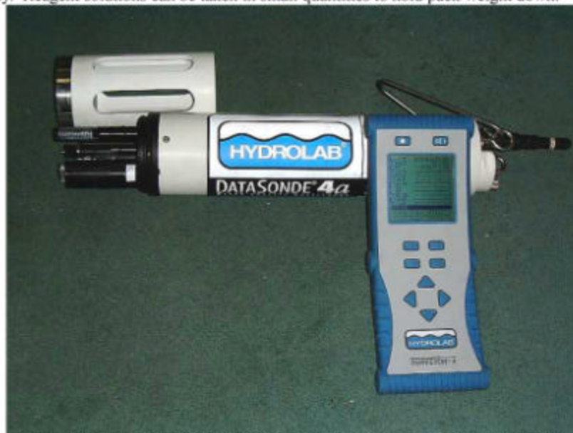
Plate 23. When necessary, greater precision can be obtained on various parameters through use of a high quality instrument, such as a Hydrolab. Packing gear of this volume and weight is generally not practical for single individuals, unless water quality information is the primary objective.
