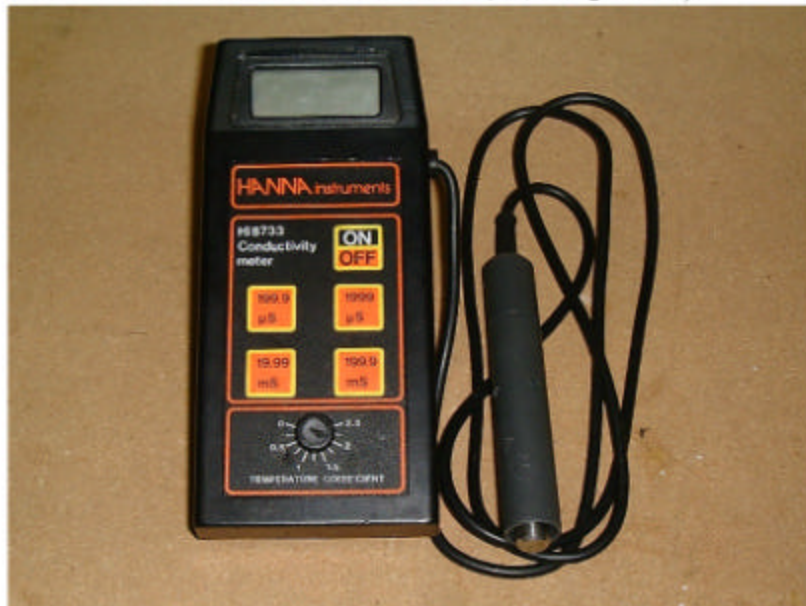
Plate 21. Conductivity readings of adequate precision can be taken with a light-weight, portable unit that is easily packed. The unit is calibrated at the beginning of each season with a highly buffered stock solution of known conductivity.
