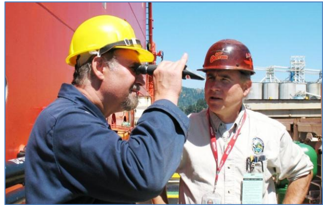
Figure 3. WDFW ballast water inspector (right) showing vessel crew how to measure salinity levels in ballast tank. WDFW photo
