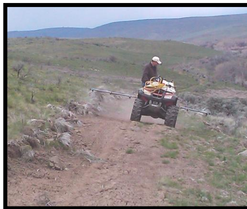
Figure 15. ATV sprayer with a 12-ft boom, spraying fire lines in Yakima County
