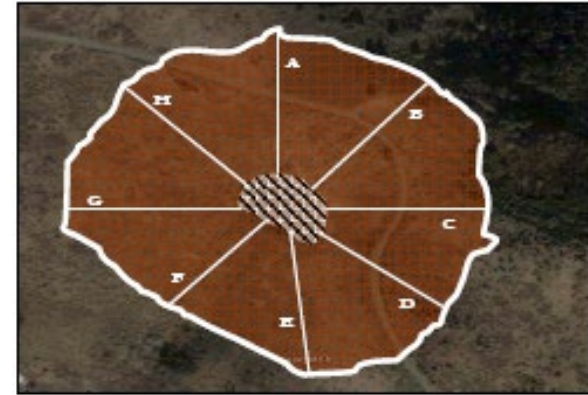
Figure A13. Transects drawn at regular intervals that are extending 250 m from the outer edge of an AA.
