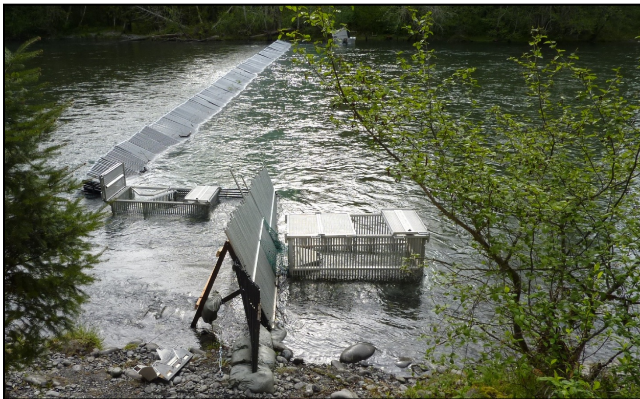
Figure 7. The winter 2011 trapping configuration used three traps: One upstream trap and one downstream trap on river left (west) bank, and one upstream trap on river right (east) bank.
