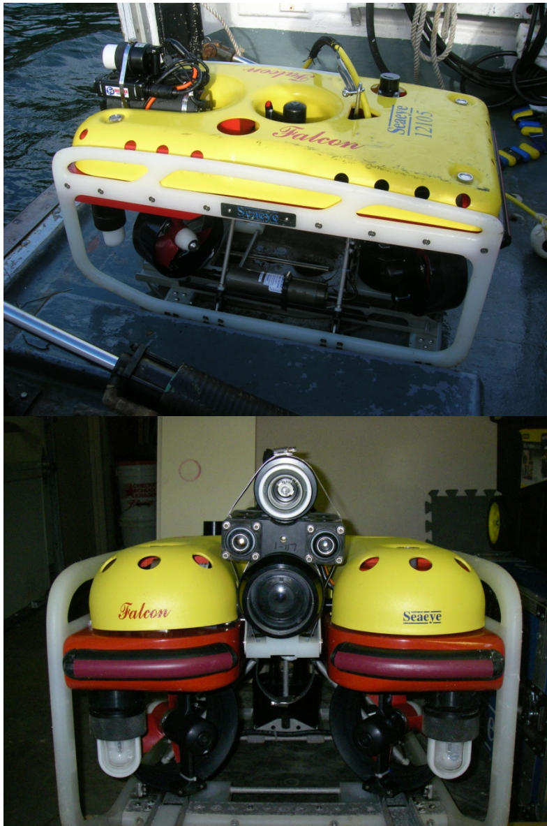
Figure 3. The SeaEye Falcon ® ROV equipped with parallel lasers.
