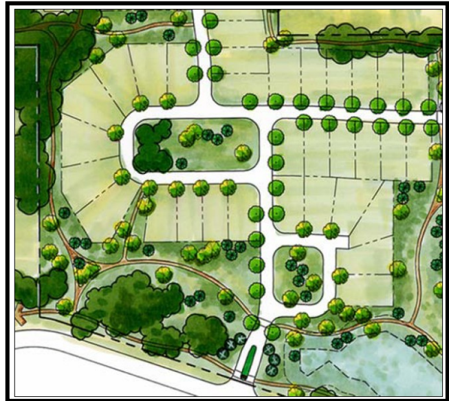
A schematic illustrating the use of a loop road design in a subdivision. This design improves safety access, and has an added benefit of enhanced stormwater management with integrated bioretention. (Source: LID Technical Guidance Manual for Puget Sound, December 2012)
