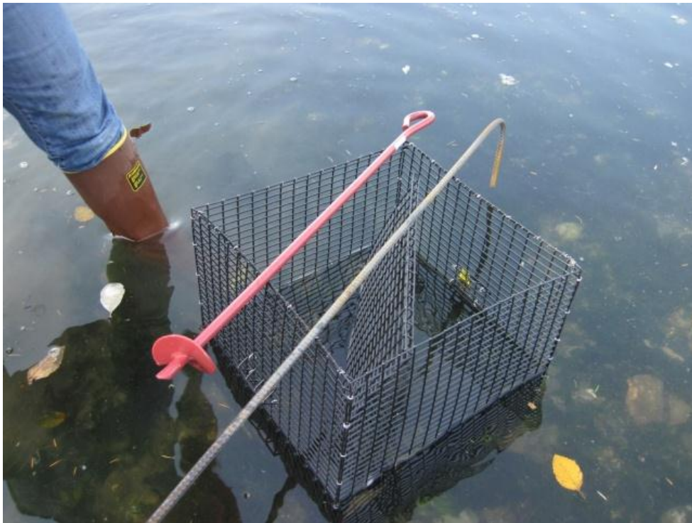
Figure 1 Cage system. Cubic cage measuring 40.6 cm (16") on a side with lid (inside cage); screw anchor measuring 76.2 cm (30 inch); bent-tip rebar measuring approximately 1.2 m (4 foot).
