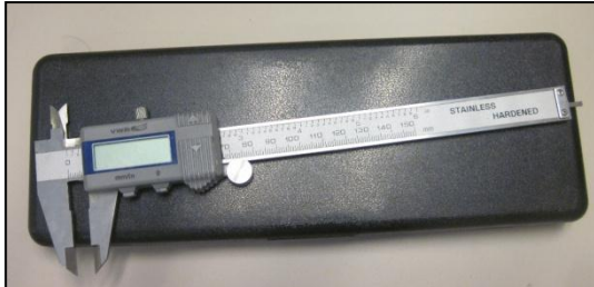
Figure 11. Stainless steel caliper with digital readout to 0.01 mm.
