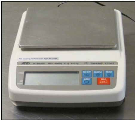
Figure 15. 6-kg capacity bench scale for weighing small specimens.
