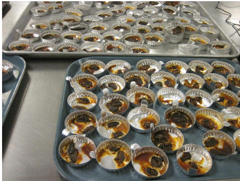
Figure 20. Mussel soft tissue after drying in a 120° C oven for a minimum of 18 hours.
