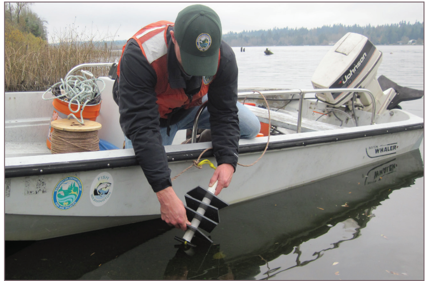
A WDFW employee uses an artificial substrate to check for zebra/quagga mussels in Lake Washington.
