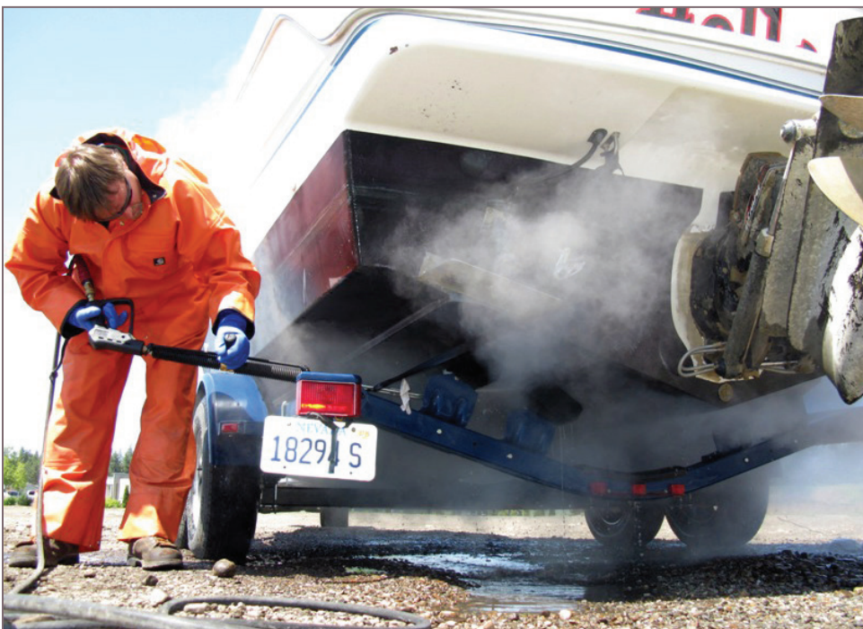
An AIS-infested boat is decontaminated in Spokane using a hot-water pressure washer.
