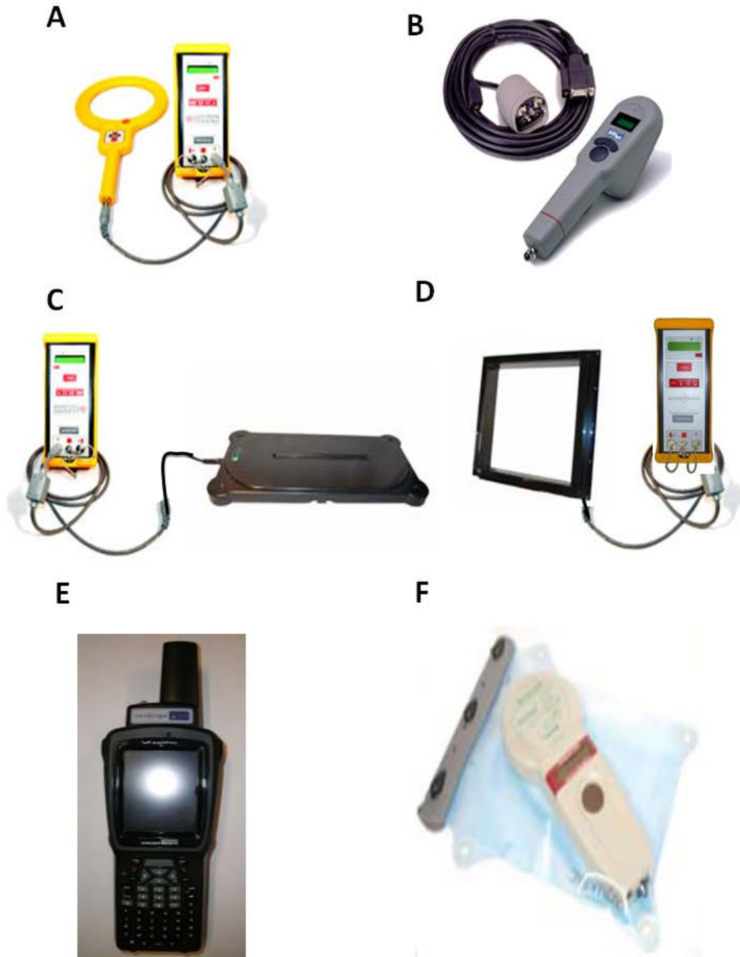
Figure 1. Picture of PIT tag detection antennae used in this study include a) Destron Fearing (DF) FS2001F-ISO Reader Base Unit (DF) with racquet, b) All Flex (AF) Model RS601-3, c) Destron Fearing (DF) FS2001F-ISO Reader Base Unit (DF) with Flat Plat (FP) antennae, d) Destron Fearing (DF) FS2001F-ISO Reader Base
