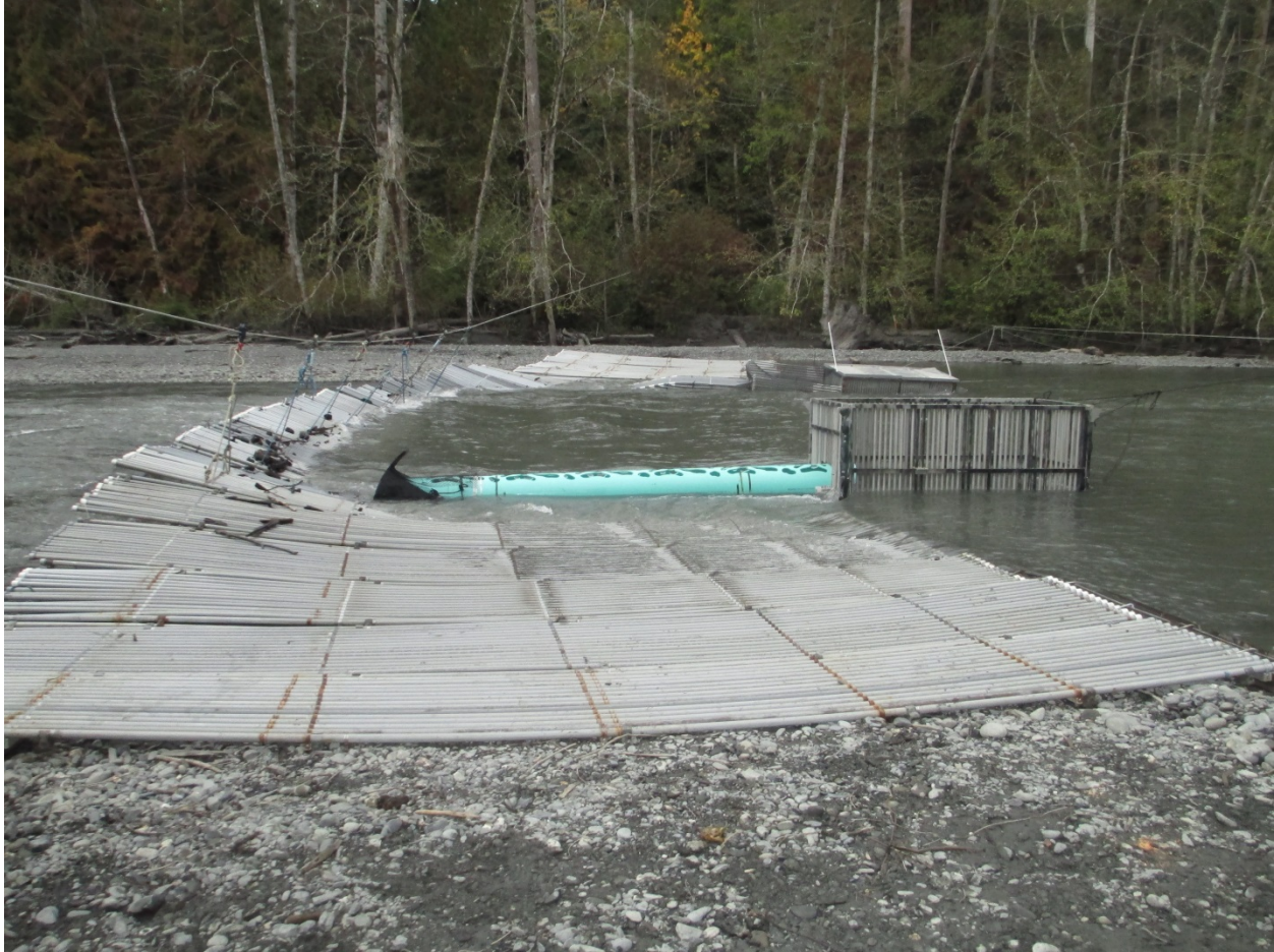
Figure 5. Experimental “pipe” trap oriented in downstream direction to capture fish moving in an upstream direction. Photo taken Aug 15 2013, discharge = 750 cfs (USGS gage 12045500), from central gravel bar looking towards right bank channel.
