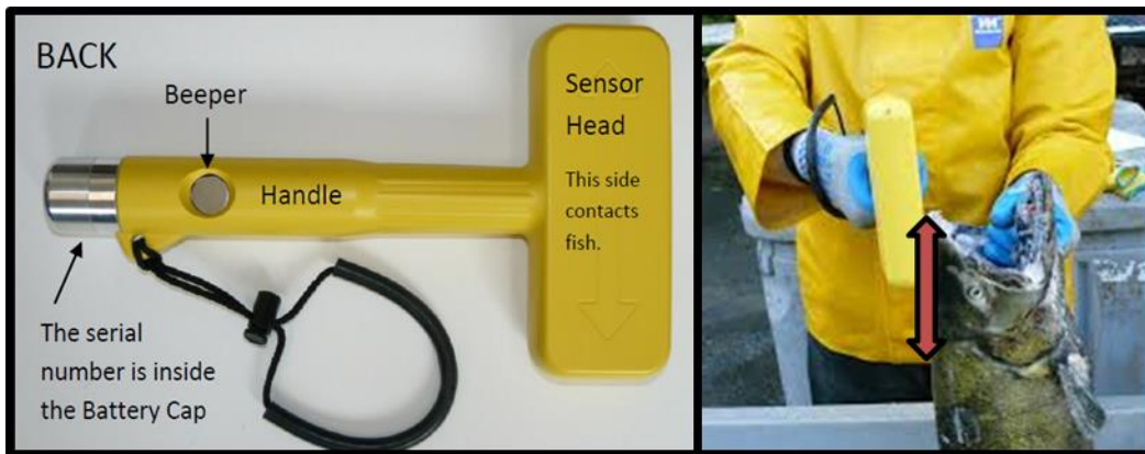
Figure 9. Location a fish should be scanned for a CWT using a “T-wand”.
