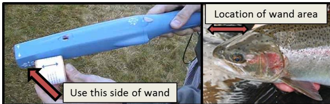
Figure 8. Location a fish should be scanned for a CWT using a “blue” wand.
