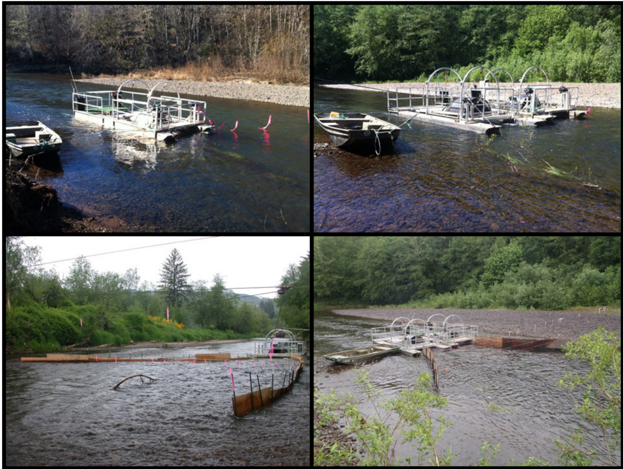
Figure 3. Grays River mainstem trapping configurations: fishing a single trap (top left), two traps fishing in tandem (top right), single trap with panels installed (lower left) and two traps fishing in tandem with panels installed (bottom right).
