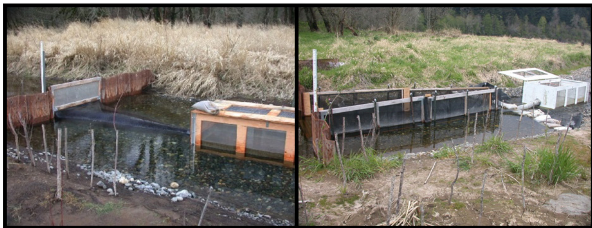
Figure 6. Duncan Creek spawning channel trapping configurations: fyke net with live box used in 2002 (left side) and fence panel weir with live box used in 2003-2016 (right side).
