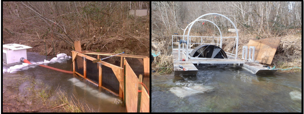
Figure 4. Crazy Johnson Creek trapping configurations: fence panel weir with live box used in 2011-12 (left side) and rotary screw trap used in 2013-16 (right side).
