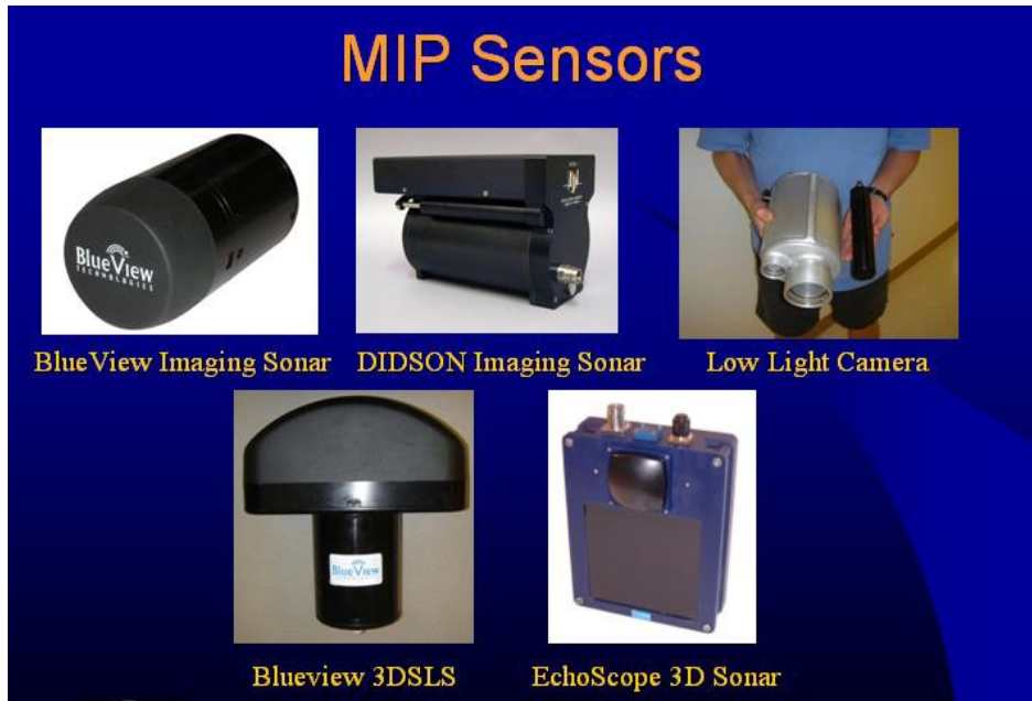
Figure 4. Mobile Inspection Package sensor suite
