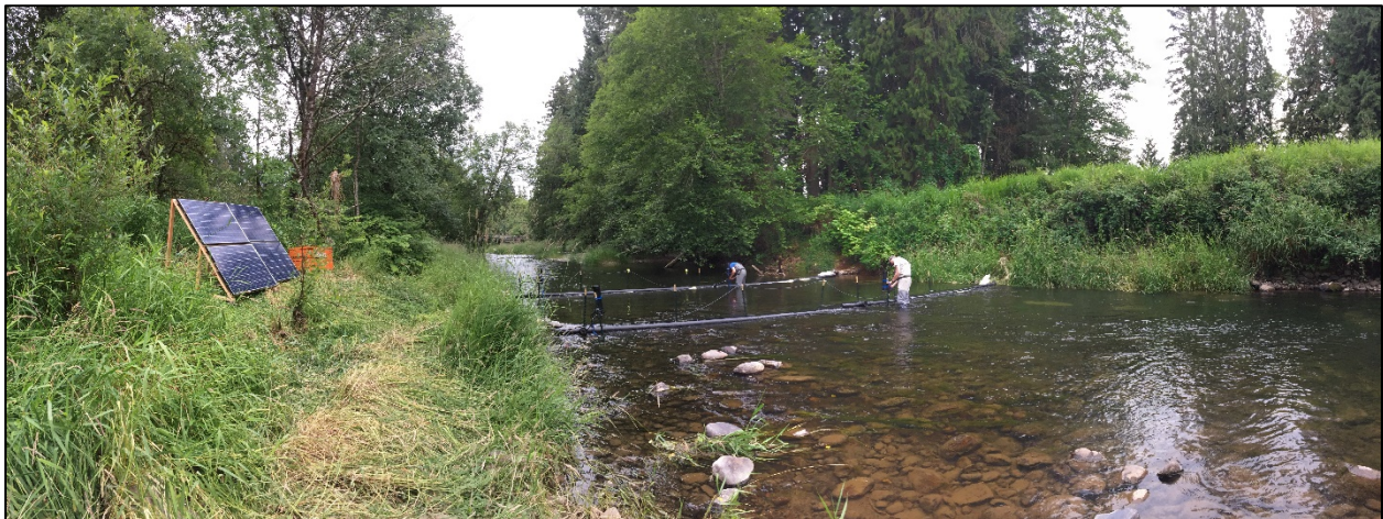
Figure 2. Passive integrated transponder (PIT) detection array (A1) in South Fork Newaukum River.
