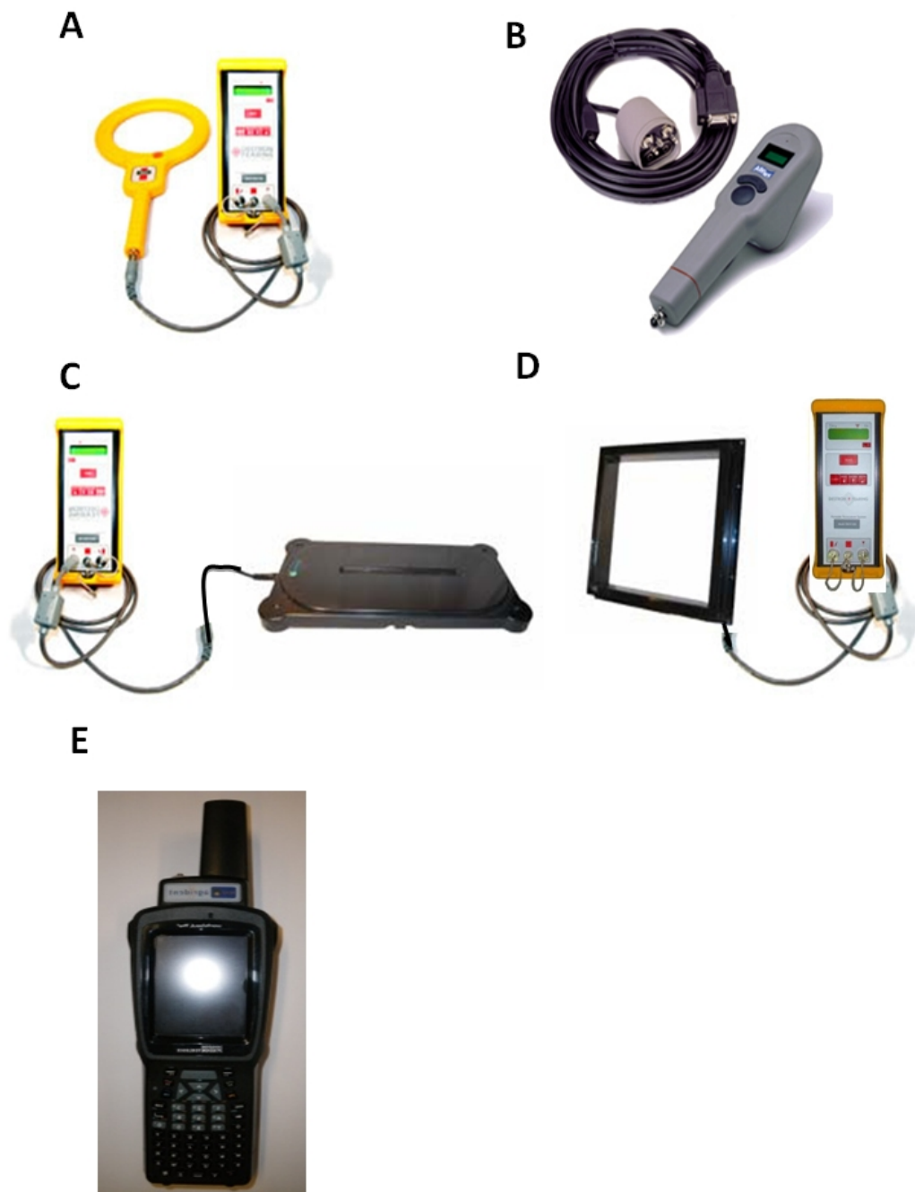
Figure 1. Pictures of PIT tag detection antennae used in this study include a) Destron Fearing FS2001F-ISO Reader Base Unit with racquet, b) Allflex Model RS601-3, c) Destron Fearing FS2001F-ISO Reader Base Unit with Flat Plat antenna, d) Destron Fearing FS2001F-ISO Reader Base Unit with 24 inch square antenna, e) Psion Teklogic data logger with RFID.
