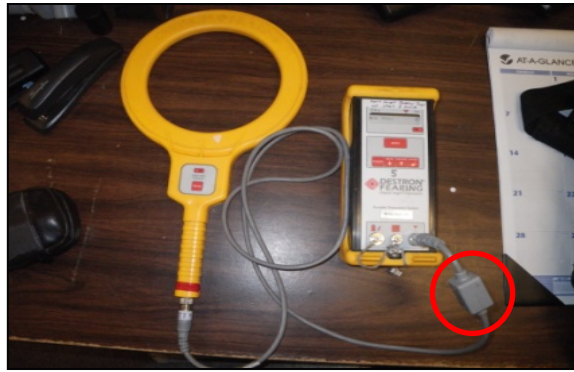
App. 1 - Figure 2: Correct assembly of the FS2001-ISO “Cheese Block”
