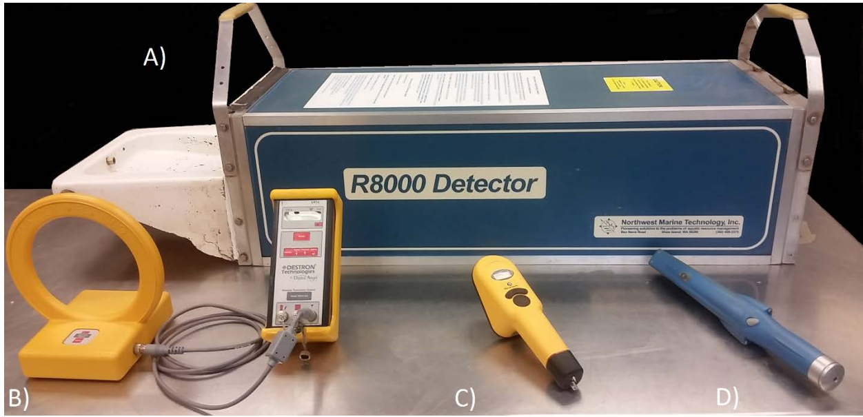
Figure 4. Tag detection equipment used by RGSP dockside samplers: A) R8000 B) Destron with tabletop antenna C) 601 Handheld reader D) Handheld CWT wand.
