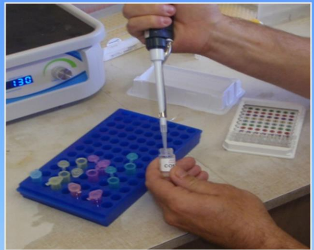
Adding domoic acid control to dilution series
