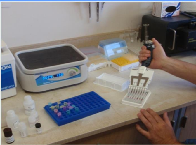
Transferring sample dilutions to a microplate
