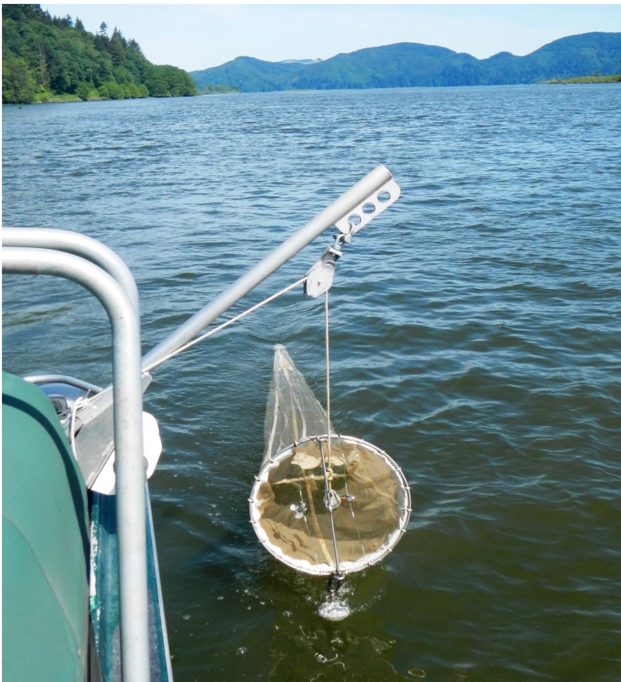
Figure 3. Photograph of the plankton net setup deployed to collect eulachon smelt eggs and larvae. Image shows the setup when two General Oceanic flow meters were mounted to the frame.
