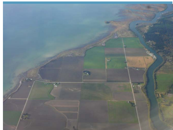
Photo 4-1 Example of delta area in which tidal barriers have restricted the river's connection to the floodplain and led to the loss of tidal wetlands (Photo courtesy of Coastal Geologic Services)
