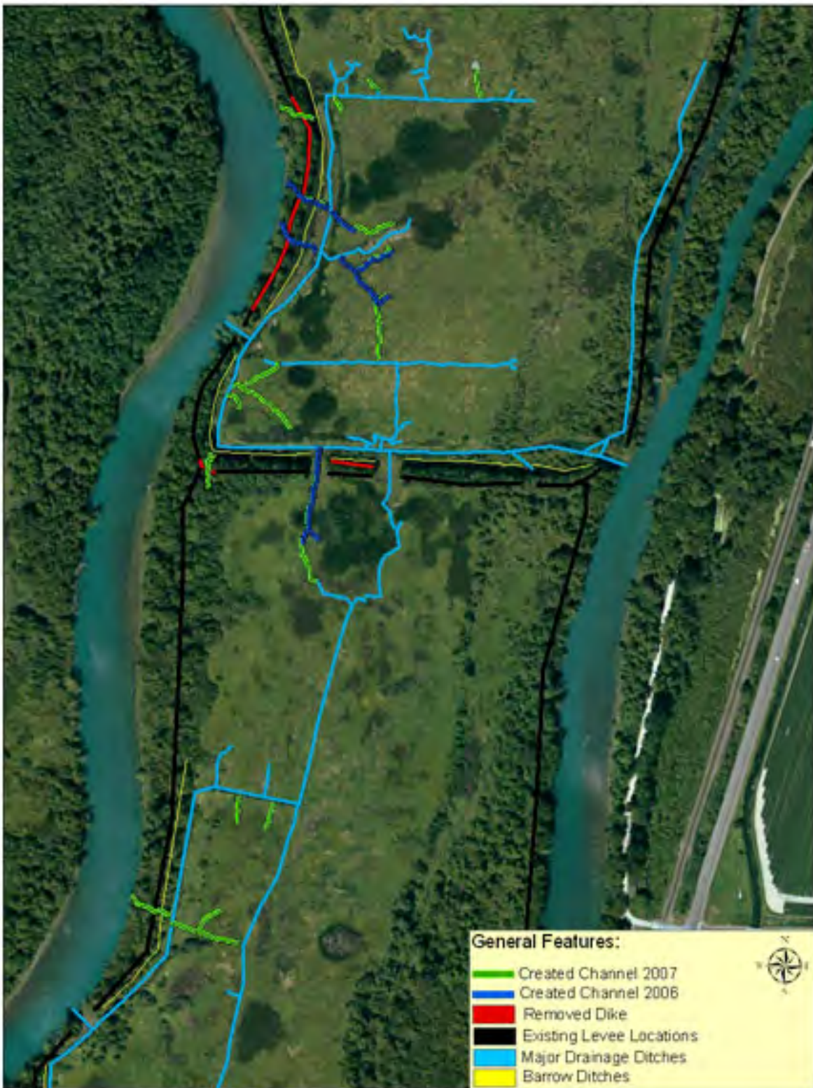
Figure 4-2 Restoration features, Milltown Island.
