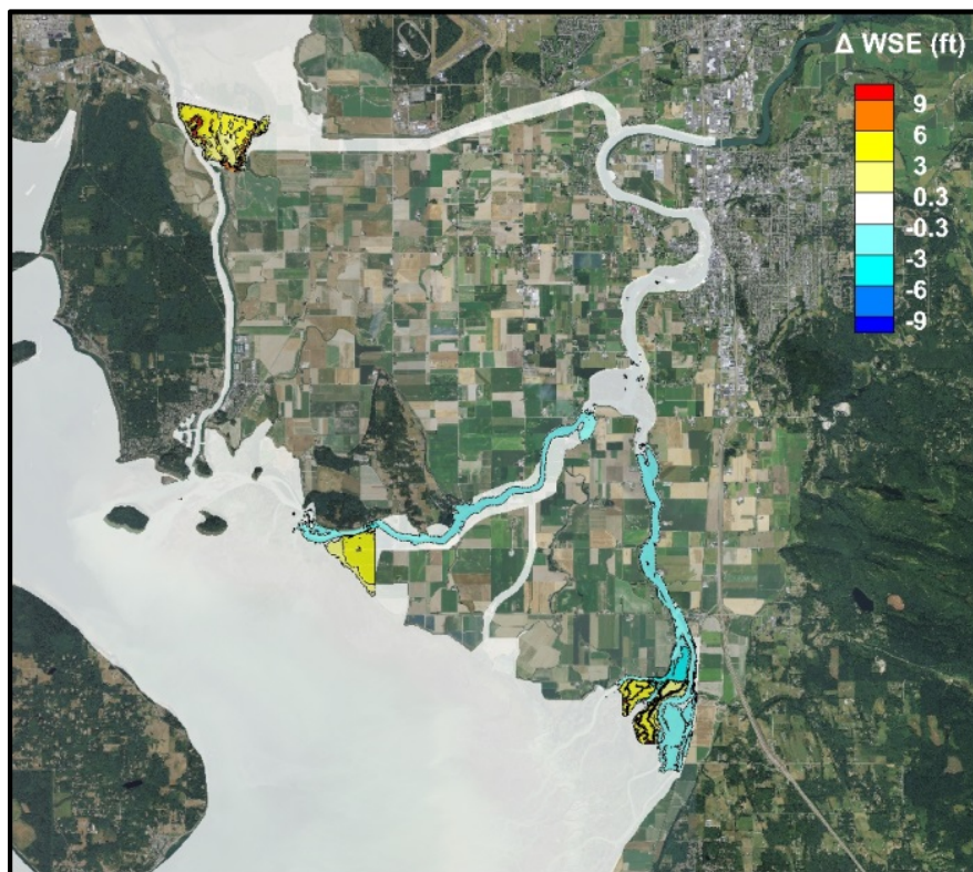
Figure 20 - Contour map of change in WSE from baseline to full restoration with flood flow in the river and high tide. (Whiting et al, 2017)
