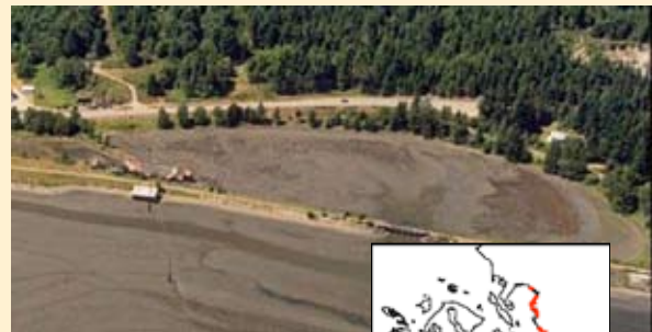
Above, South Discovery Bay, Jefferson County. Tidal restriction resulting from rail causeway. Right, Puget Sound and Northern Straits shores with railway revetments/causeways (red). (WDNR 2001).
