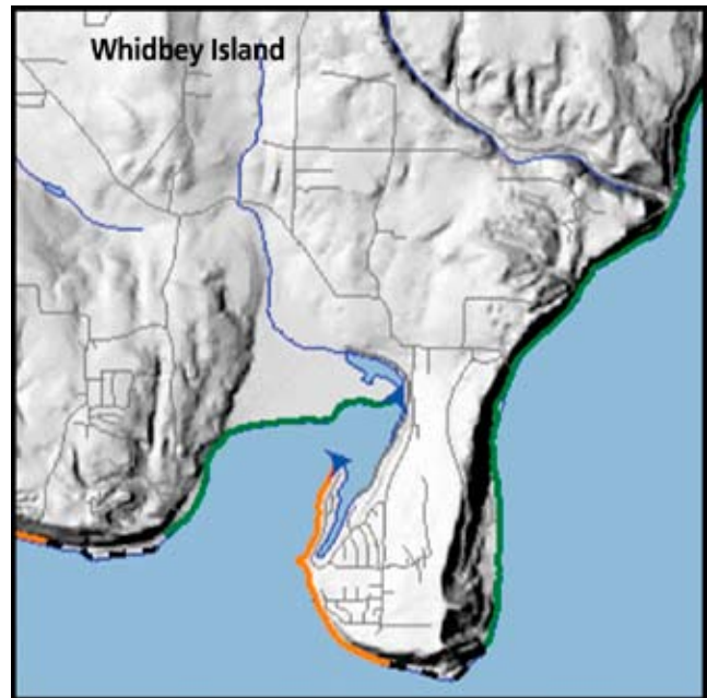
Figure 5. Example of net shore-drift cells from southeast Whidbey Island (Johannessen 1992). Presentation is from Washington Department of Ecology's Digital Coastal Atlas.
