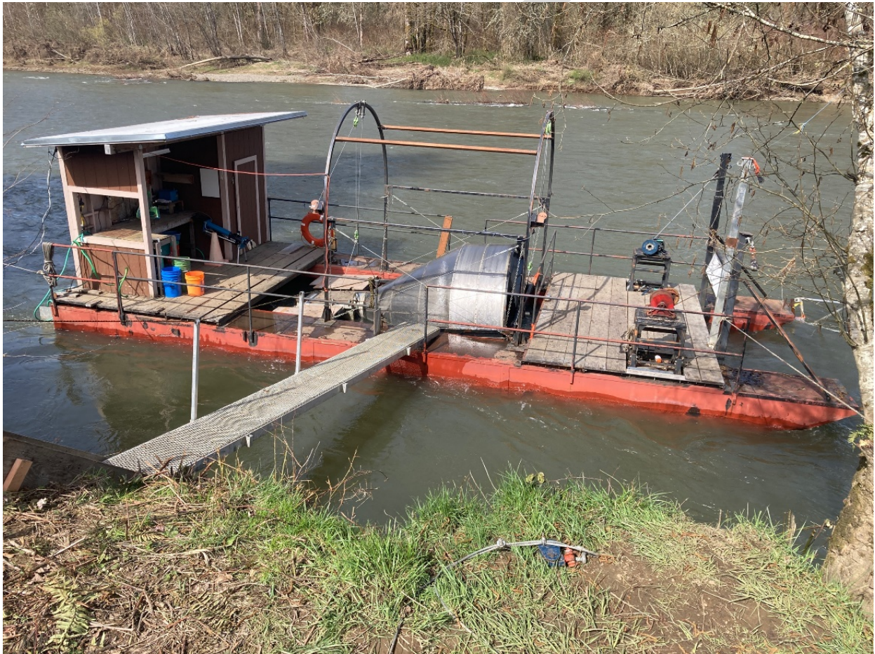
Figure 6: Rotary screw trap used to estimate juvenile steelhead abundance originating upstream of river mile 52 on the Chehalis River of Grays Harbor showing cone, livebox (covered), and floating pontoons. (Photo: D. Olson)
