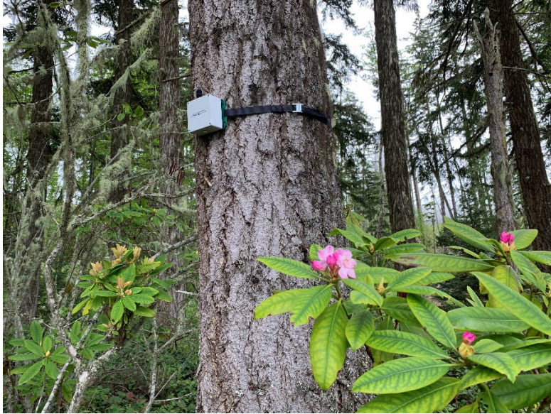
An acoustic recording unit deployed to record hooting male sooty grouse. Photo by Shelly Ament.
