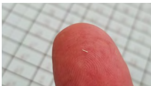
Figure 2. Coded wire tag on fingertip (WDFW)
