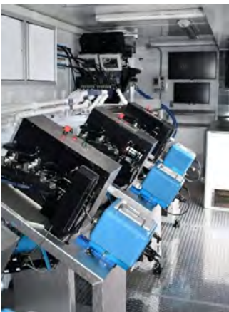
Figure 4. Computer controlled AutoFish System inside trailer containing a sorter and six marking and tagging lines. Adipose fins are clipped via black mechanisms and then CWT inserted using blue injectors.
